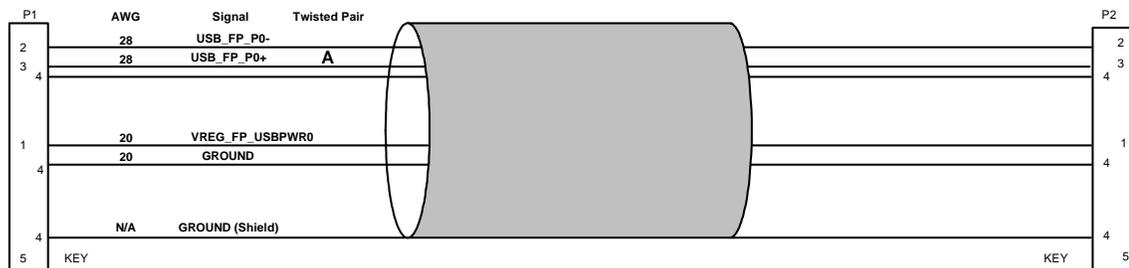
**Figure 18. Single Port USB Cable Wiring Diagram**
